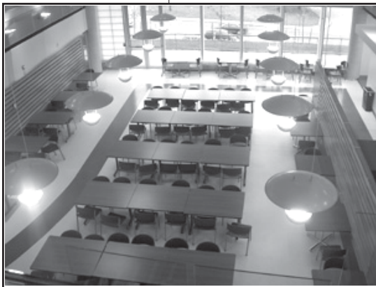
Ample natural and artificial lighting sources combine to provide a comfortable environment for all in the CNIB cafeteria. The color-contrasted and tactile flooring strip is attractive and provides a unique wayfinding cue for users with visual impairments.
