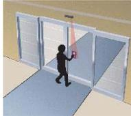
Above: Infrared light aimed at the Wave Hand sticker. When activated it expands coverage (below).
