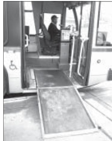
The universal ramp design of the “stairless” bus, by Nova Bus Corp., makes boarding easier for everyone.
