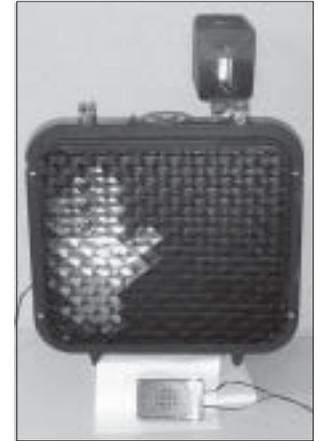
The Talking Signs transmitter, mounted on top of the pedhead. The hand-held receiver, carried by the blind pedestrian, is in front. When the receiver is aimed at the transmitter and the button is pressed, the transmitter provides information about the status of the "Walk/Don't Walk" signal. The speech message comes from the receiver, which the blind person has in his or her hand.
